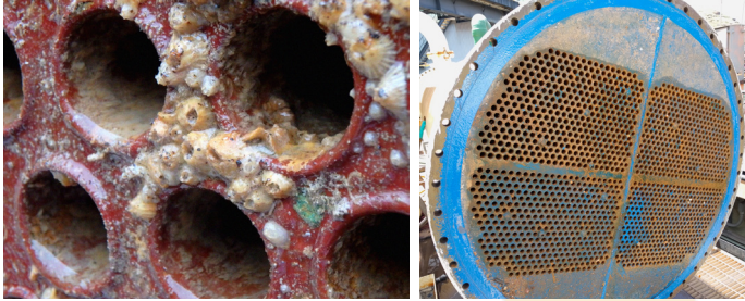
Figure 3: Untreated tubulars six months after a standard cleaning vs. HeatX-treated heat exchanger after six months in service: no maintenance was required.
